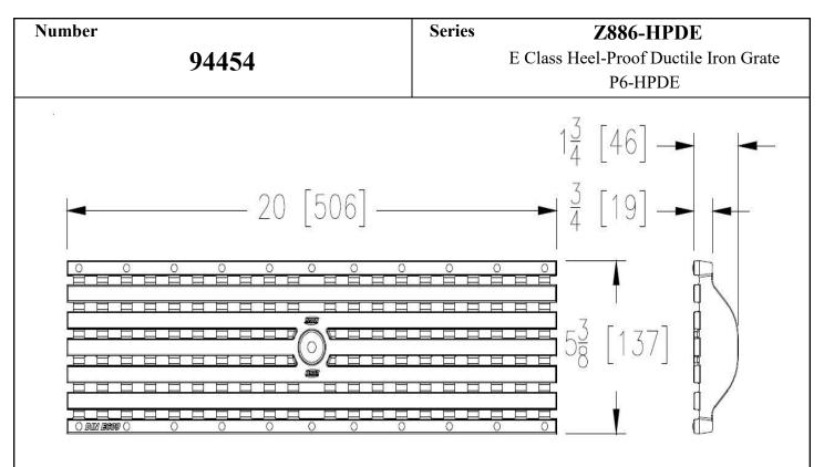
The Zurn P6-HPDE Heel-Proof Slotted, Ductile Iron Grate, is 5-3/8 inches wide by 20 inches long, weighing 9.5 lbs per linear foot. The grate has an open area of 22.2 square inches per linear foot, DIN Rating of E, ANSI Rating of Special-Duty, ADA compliant, H-20 Load Rated and FAA Load Rated. Supplied by Trench Drain Supply.
