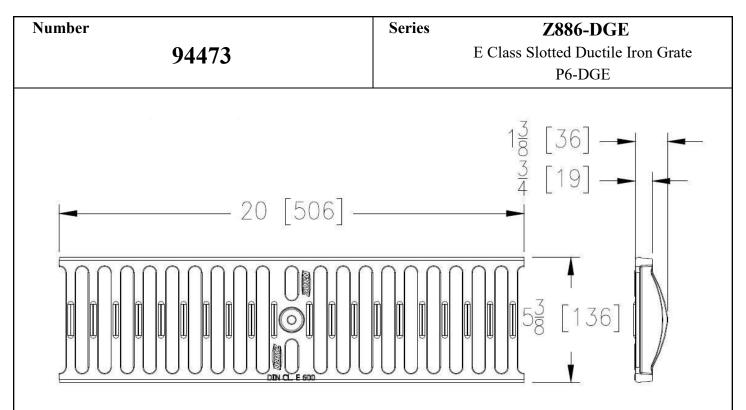
The Zurn P6-DGE Slotted Grate, Ductile Iron Grate, is 5-3/8 inches wide by 20 inches long, weighing 6.4 lbs per linear foot. The grate has an open area of 27.8 square inches per linear foot, DIN Rating of E, ANSI Rating of Special Duty, H-20 Load Rated, FAA Load Rated. Supplied by Trench Drain Supply.
