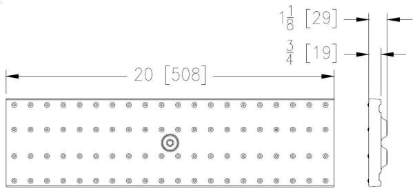
The Zurn P6-DC Solid Cover, Dura-Coated Ductile Iron Cover, is 5-3/8 inches wide by 20 inches long, weighing 8 lbs per linear foot. The grate has a DIN Rating of C, ANSI Rating of Heavy-Duty, H-20 Load Rated, ADA compliant. Supplied by Trench Drain Supply.
