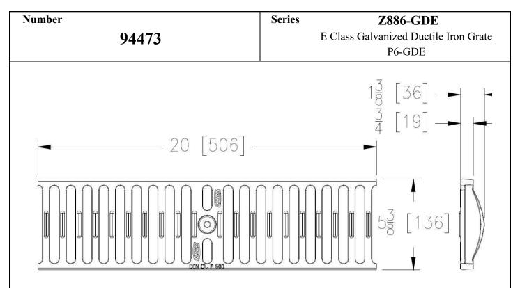
The Zurn P6-GDE Slotted Grate, Galvanized Ductile Iron Grate, is 5-3/8 inches wide by 20 inches long, weighing 6.4 lbs per linear foot. The grate has an open area of 27.8 square inches per linear foot, DIN Rating of E, ANSI Rating of Special Duty, H-20 Load Rated, FAA Load Rated. Galvanizing (Hot dip) conforms to ASTM specification A123. Supplied by Trench Drain Supply.
